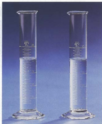
Figure 2.11a) 20 mL of rubbing alcohol and 20 mL of water in separate 25-mL cylinders
