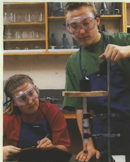
Figure 3.15 Step 7. Be sure to follow safe work procedures. Clamp the syringe tightly at right angles to the stand.
